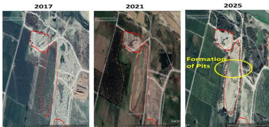
Figure 3.14 Time Series of images Showing formation of pits with time
